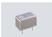
CR-338 HIGH STABILITY CRYSTAL UNIT Contains a temp. compensating heater for improved frequency stability. Frequency stability: ±0.5 ppm
